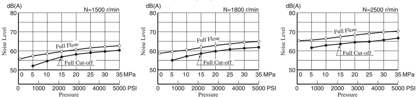
Typical Performance Characteristics of Type "A3H37" at Viscosity 32 mm<sup>2</sup>/s (150 SSU) [ISO VG32 oils, 40°C (104°F)]
