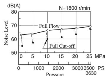
Typical Performance Characteristics of Type "A90" at Viscosity 32 mm<sup>2</sup>/s (150 SSU) [ISO VG32 Oils, 40°C (104°F)]
