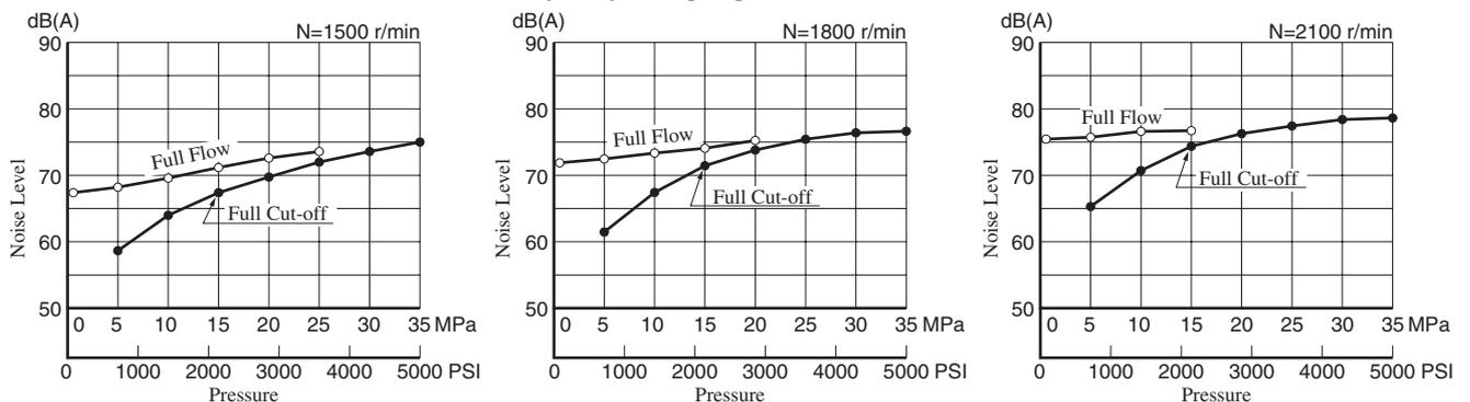
Typical Performance Characteristics of Type "A3H145" at Viscosity 32 mm<sup>2</sup>/s (150 SSU) [ISO VG32 oils, 40°C (104°F)]
