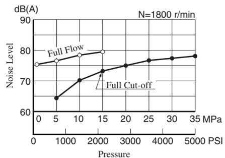
Typical Performance Characteristics of Type "A3H180" at Viscosity 32 mm<sup>2</sup>/s (150 SSU) [ISO VG32 oils, 40°C (104°F)]
