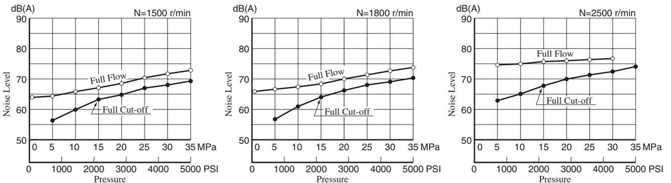
Typical Performance Characteristics of Type "A3H71" at Viscosity 32 mm<sup>2</sup>/s (150 SSU) [ISO VG32 oils, 40°C (104°F)]
