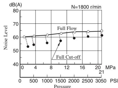
Typical Performance Characteristics of Type "A22" at Viscosity 20 mm<sup>2</sup>/s (100 SSU) [ISO VG32 Oils, 50°C (122°F)]
